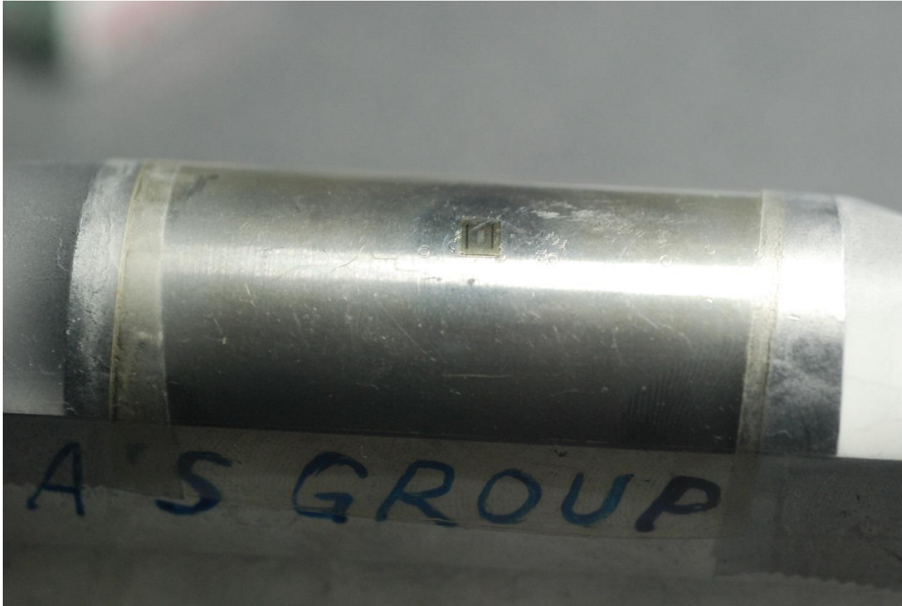
Figure S3. Camera Image of transparent graphene/AlGaIn with embedded GaN 2DEG released and transferred on PET Film with bending radius=18.5mm.
